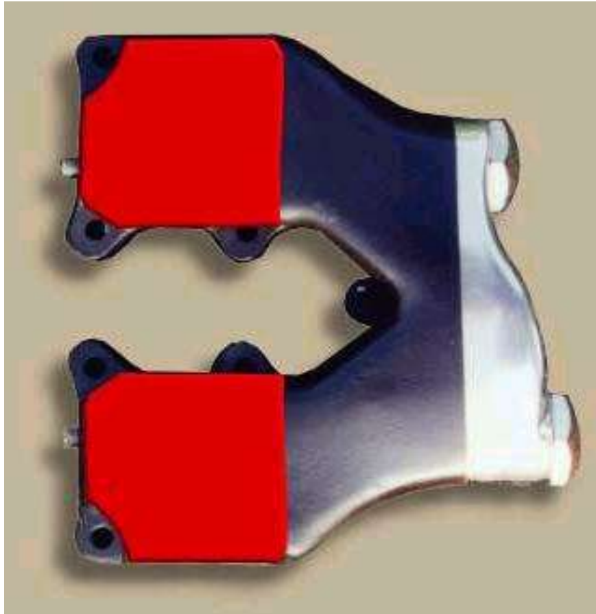
Figure 4 Highlighted areas show the areas which can be modified. Take down material by mill or sharpen
