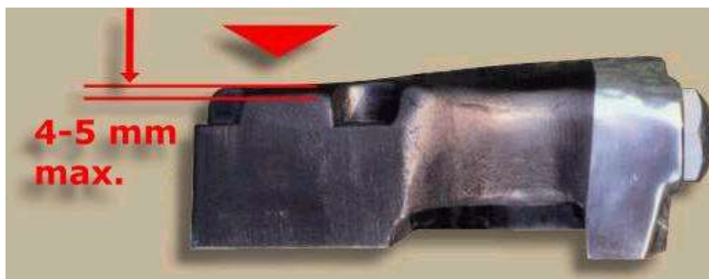
Figure 3 At the back top side of the Knovelhead rockerbox you can cut at most up to 5 mm of materia.
